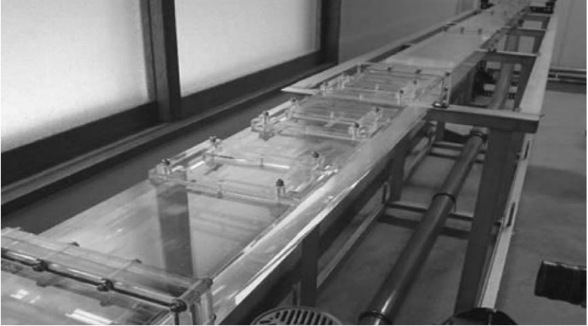
Figure 2 Horizontal channel for the gas–liquid two-phase flow experiments.
